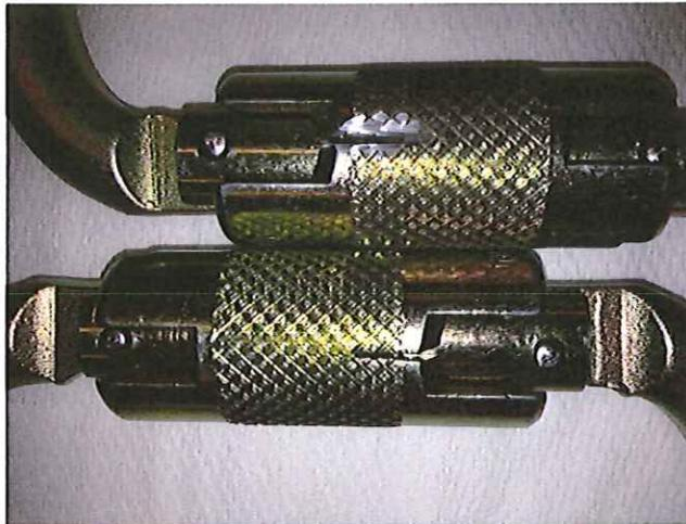
The attached picture shows two of the same type of carabiner (P/N 10089207). The bottom gate is normal. The top one has had some of the knurling ground off in order to show the full width of the machined slot.
